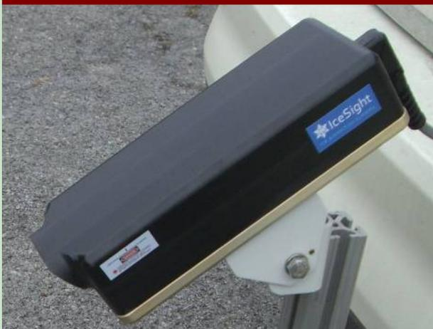
Mobile **IceSight** scans the road surface for hazardous driving conditions. The flexible data stream can be integrated with existing telematic systems for easy data transfer or sent to a hand-held device or lap-top for real-time monitoring.
