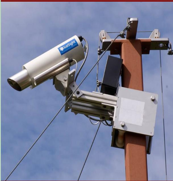
**IceSight** uses infrared technology to detect hazardous Ice, Snow, Slush, or Wet pavement conditions. Information is uploaded to DOT networks. It can also be integrated with roadside warning signs or can activate embedded sprayers to disburse liquid anti-ice chemicals on road and bridge surfaces.
