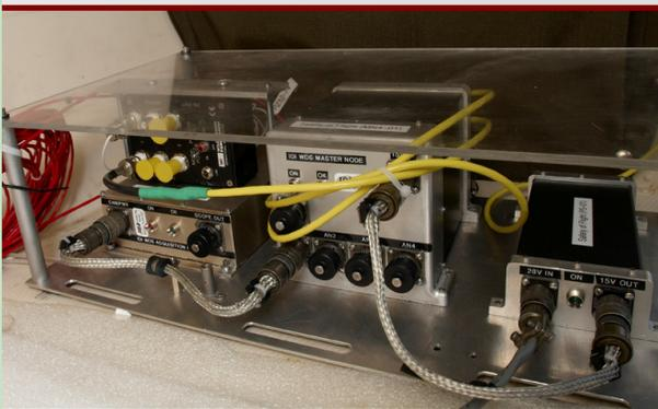
In-situ aircraft **Wiring Sensor System** for monitoring precursor damage such as wire chafing. Size, weight and power are key attributes for aircraft deployment.
