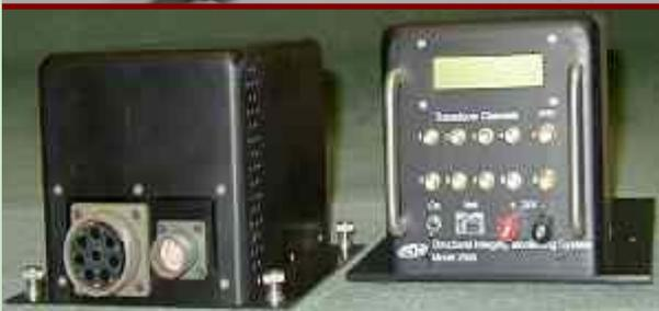
**Structural Integrity Monitor** for assessing the health of aircraft structures using a network of distributed piezoelectric actuators and sensors.
