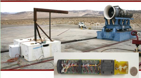
Self-powered 8-channel wireless transmitter for measuring **Temperature and Strain** on rotating machinery. The device was used to monitor a TF-41 fan disk at China Lake in support of FAA research into engine failure modes.
