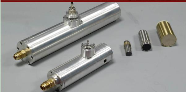
**Fluid Debris Sensor** mounted in-line through the pipe wall perpendicular to the flow focuses ultrasound energy into the fluid. Particles within the focal region reflect the energy generating echoes proportional to the particle size.
