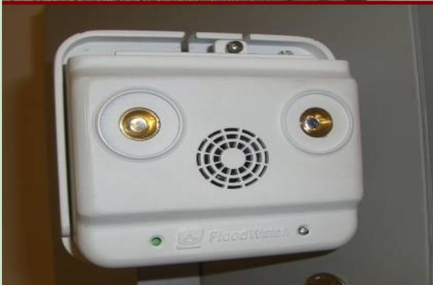
**FloodWatch** is a non-contact ceiling mounted infrared sensor protecting the home owner from catastrophic floods.
