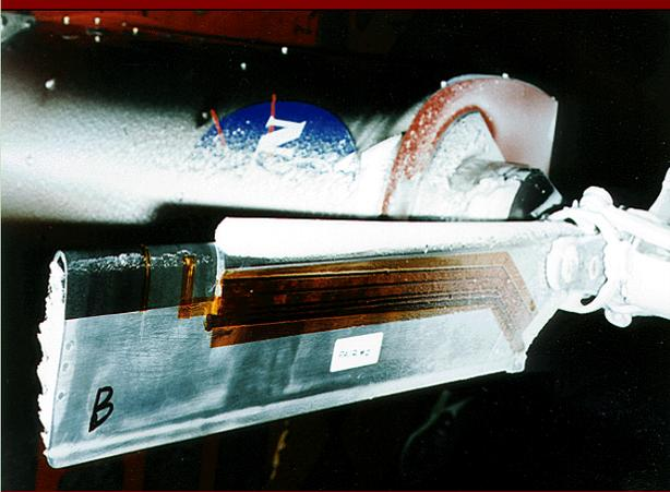
**Shape Memory Alloy Deicer** mounted on powered rotating rig in NASA Glenn's Icing Tunnel.
